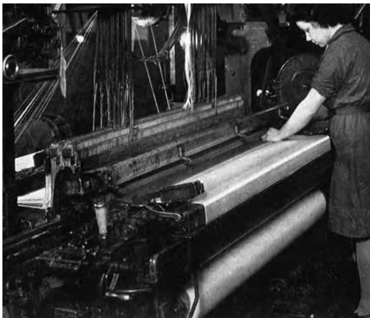
PLATE 7 Weaving: the healds lift and lower sections of the warp creating the shed through which the shuttle flies. This interlacing of warp and weft constructs the cloth
