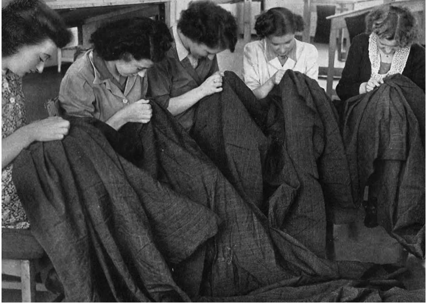
PLATE 8 Mending: girls rectify small faults that have occurred in the weaving
