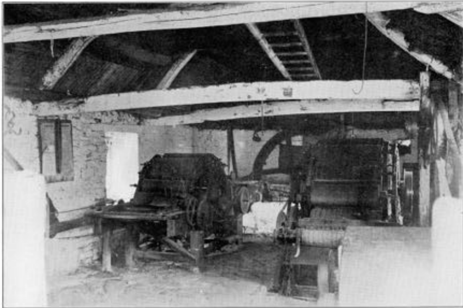
Fig. 7. Llanrhystyd Woollen Yarn Factory. Interior showing the scribbler-carding machine (left) and the condenser-carding machine (right) with the willy in the foreground (right).
