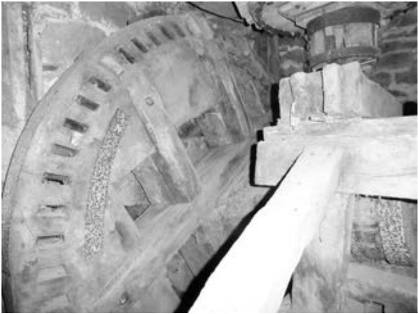
PLATE 5 The clasp-armed wooden pitwheel
